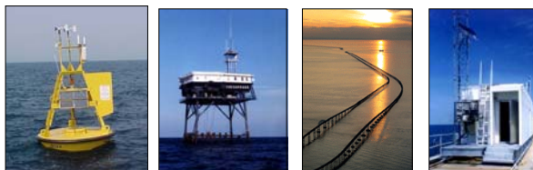
Buoy 44014 - Located at 64 nm East of Virginia Beach. Is a NOAA 3 meter discus buoy anchored on 47.5 m water depth. The anemometer height is 5 m above sea level.
