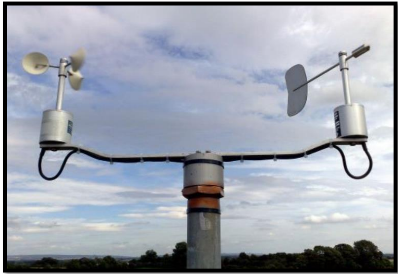
Cup Anemometer (speed & direction at 10m)
